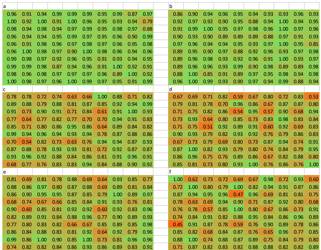
Fig. 3. Set of DoH matrices obtained every 15 days after the Round-Robin tests carried out on the aluminum structure, from (a) initial state to (f) final state.
