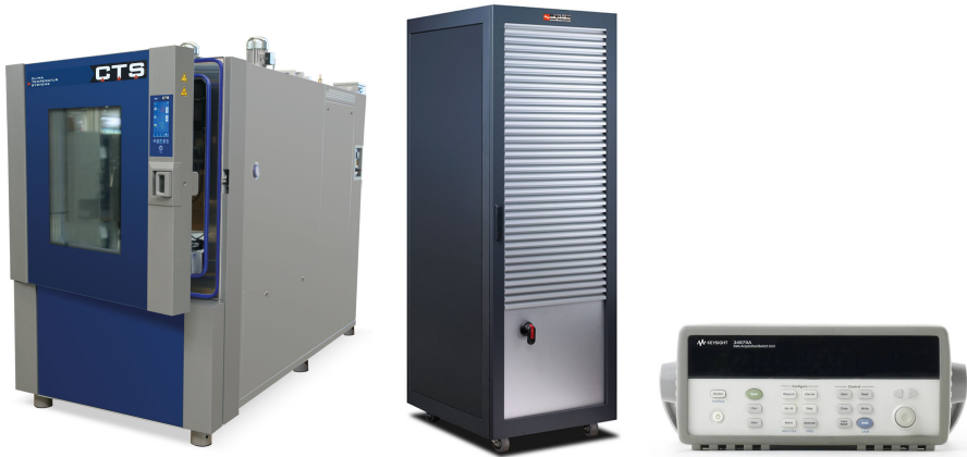
(a) Thermal Chamber (CTS). (b) Programmable Cycler. (c) Data Acquisition System (DAQ).
