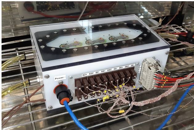
Figure 6.10: Dielectric flow- and tab-based prototype experimental test setup.
