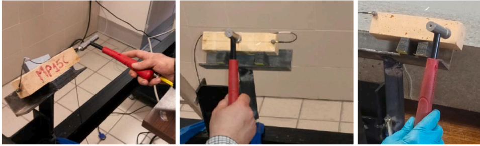
Fig. 4. Tests conducted at the laboratory, (a), longitudinal mode of vibration, (b) transverse mode of vibration, and (c) torsional mode of vibration.
