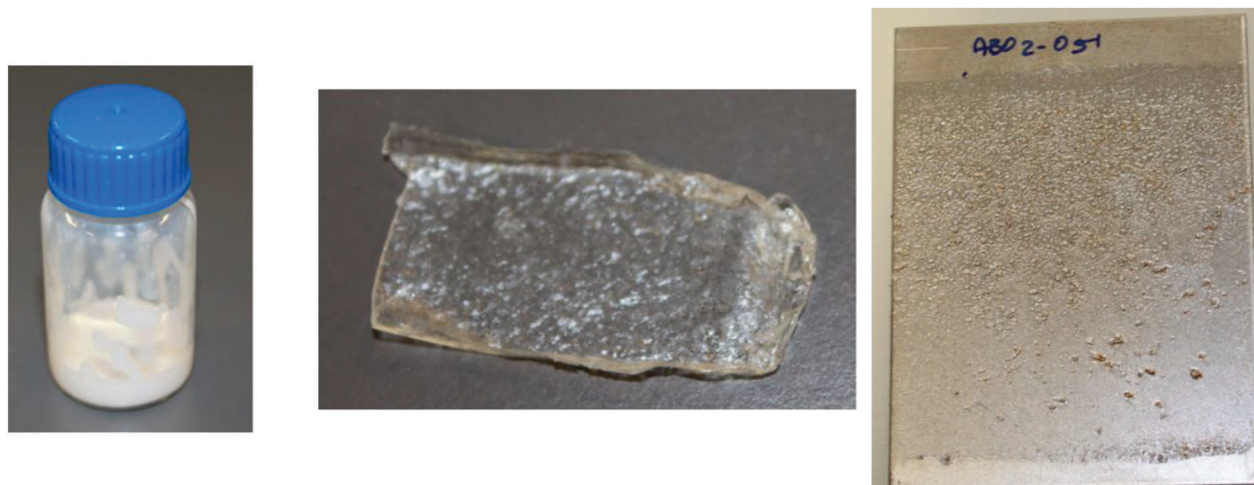
Figure 3. Picture of the latex (left), self-standing film (middle), and a film on the steel substrate of the PU/acrylic hybrid obtained using a phosphate macrodiol in the synthesis of the PU prepolymer.
