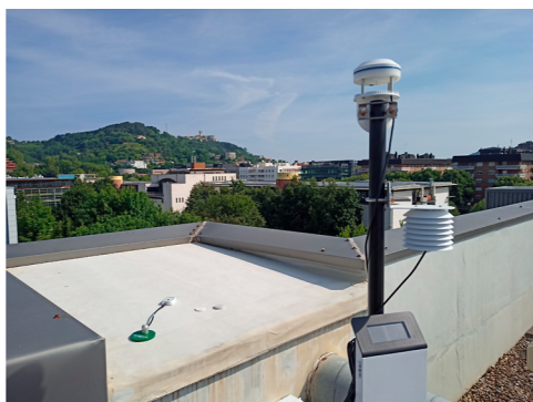
Figure 2. Prototype for assessing cooling performance under solar radiation.
