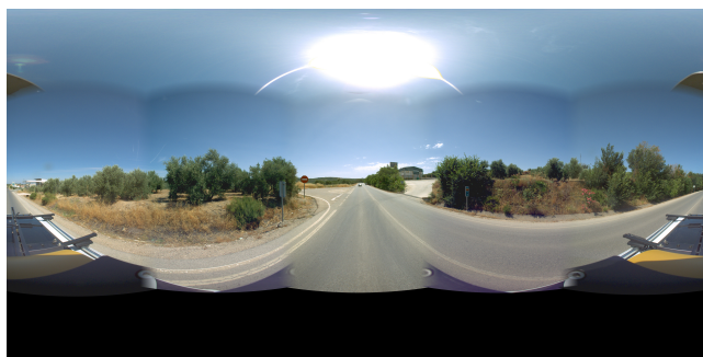
Figure 2: An example panorama from the ladybug sensor, obtained by the composition of the views of the five cameras.
