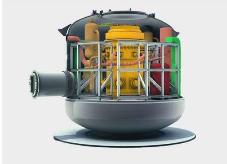
Figura 1 Diseño general del reactor NUWARD con la vasija y el recipiente exterior de acero [Ref. <https://world-nuclear-news.org/Articles/French-developed-SMR-design-unveiled>]
