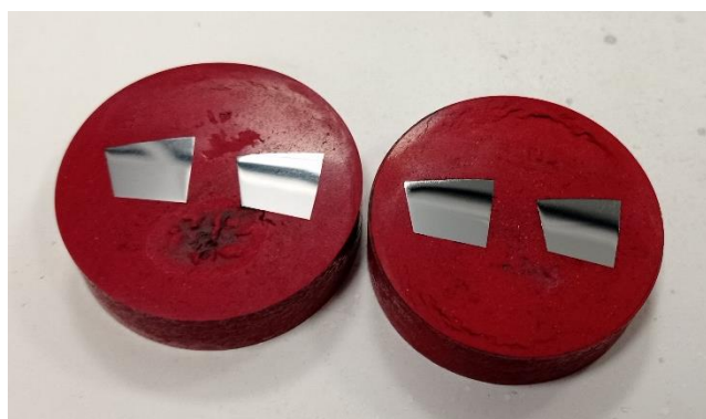
Figure 62. A mirror finish is achieved after the polishing process.
