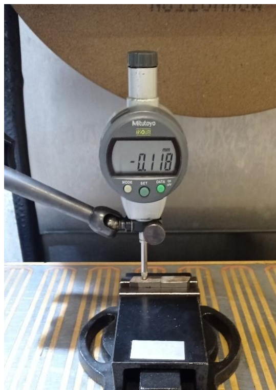
Figure 55. Measuring the real grinding total depth of cut with a dial indicator.
