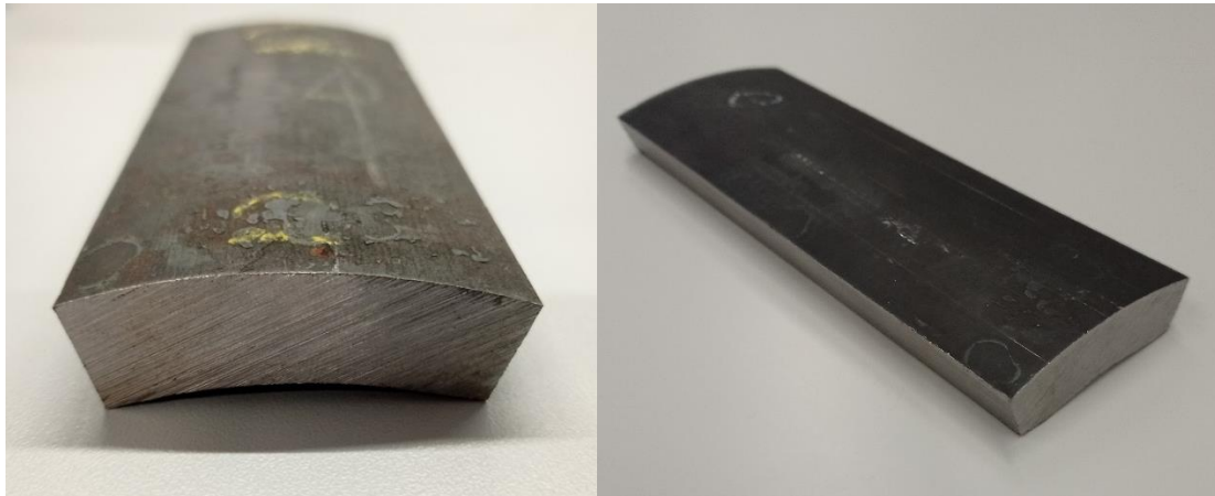
Figure 33. API 5L X70 steel pipe segment from which specimens were taken for the grinding tests of this project.
