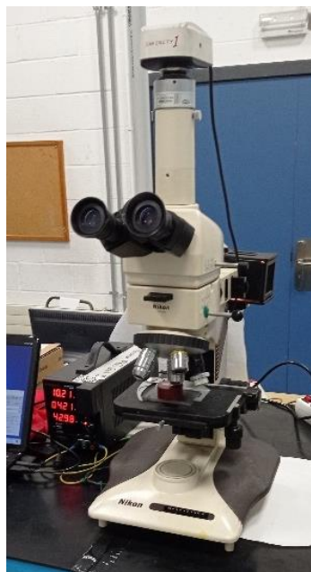
Figure 44. NIKON Optiphot-100 optical microscope equipped with the INFINITY1 digital color microscopy camera.
