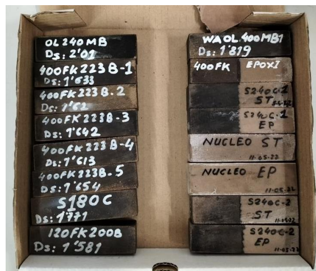
Figure 69. Various specimens of different compositions prepared for three-point bending tests.
