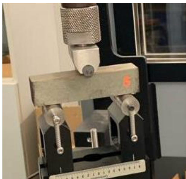
Figure 71. Three-point bending test of a sample of abrasive compound.
