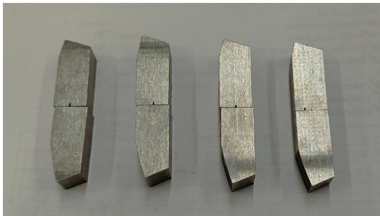
Figure 52. Four specimens ready for installing the thermocouples and performing the grinding tests.
