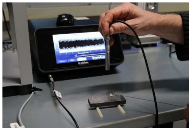
Figure 10. Using the Grindo Sonic testing equipment to determine the mechanical properties of a metal sample. Source: UK Atomic Energy Authority.
