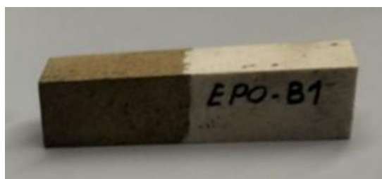
Figure 70. Mix specimen composed of abrasive material (left side) and resin core material (right side). The grooves to improve the adhesion between both materials can be noticed in the upper surface.
