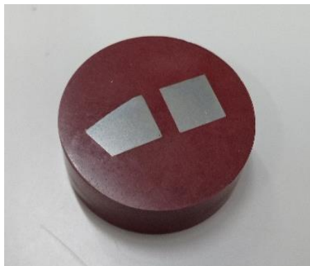
Figure 63. A matte finish is achieved after etching the polished specimens.
