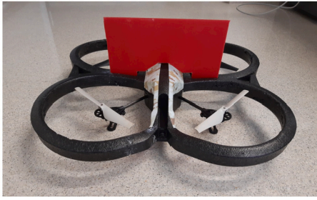
Fig. 1. UAV with the red card mounted. (For interpretation of the colors in the figure(s), the reader is referred to the web version of this article.)
