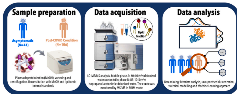
Fig. 2. Workflow of the untargeted lipidomics approach: 147 plasma samples from PCC patients were deproteinized using LC-MS-grade MeOH, vortexed, and centrifuged. The supernatant was reconstituted with MeOH and a lipidomic internal standards mix, vortexed, and analyzed. The LC-MS/MS analysis used positive or negative MRM detection mode. Mobile phase A was 60:40 (v/v) water:acetonitrile, while phase B was 85:10:5 (v/v) isopropanol:acetonitrile:water. The chromatographic eluates were monitored by MS/MS in MRM mode. Data analysis involved bivariate analysis, unsupervised clusterization, statistical modeling, and ML. A Multinomial Regression model with logit link was used to classify and understand lipidomic differences between PCC groups and asymptomatic patients. Additionally, a Random Forest model analyzed the classification based on lipidomic concentrations.
