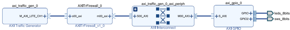
Fig. 8. Vivado block diagram of the evaluation testbed. AXI master, AXI Firewall, and AXI Slave (GPIO) — with required AXI interconnect and other AXI infrastructure cores.
