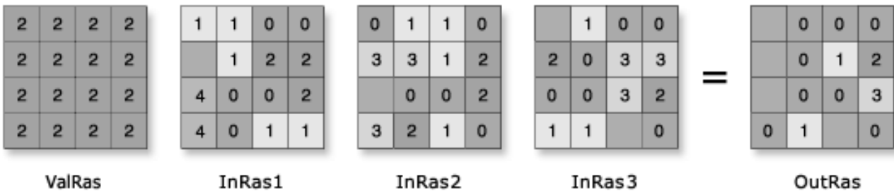
FIGURE 3: SCHEMA OF THE EQUAL TO FREQUENCY TOOL CALCULATION PROCESS (IMAGE: ARCGIS HELP 10.1).
