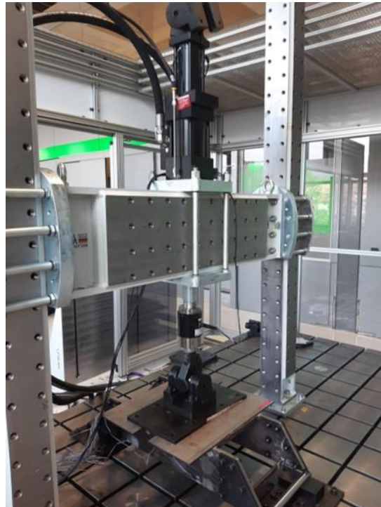
Figure 3. Use case and implemented scenario: scaled prototype of a bed of an industrial press installed in the fatigue test machine.
