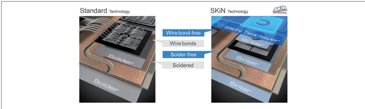
Fig. 5: Comparison of standard connection technology and SKIN technology. Picture is from [4]
