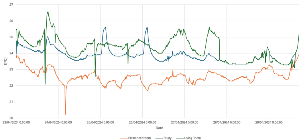
FIGURE 36. MEASURED INDOOR TEMPERATURE OF THREE ROOMS FROM 23 RD OF APRIL UNTIL 29 TH OF APRIL.
