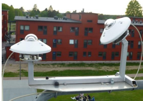
Figure 20 Pyranometers in building 45 measuring total radiation in a horizontal surface and in a tilted surface
