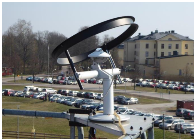
Figure 21 Pyranometer with a shading ring taking diffuse radiation
