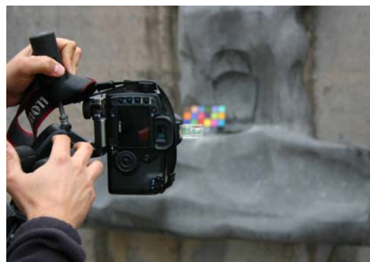
Figure 1: Color chart added in the scene so as to be able to compare its radiometry in a temporal sequence.
