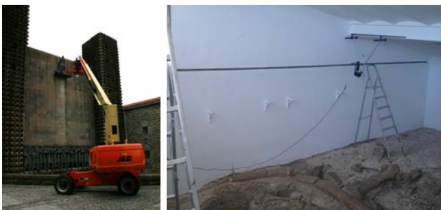
Figure 2: Auxiliary equipment to take the photographs under an optimal geometry: a crane (left) and metallic bars (right).
