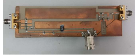
Fig. 5. Photograph of frequency divider fabricated in hybrid technology using an SMV1255 varactor.
