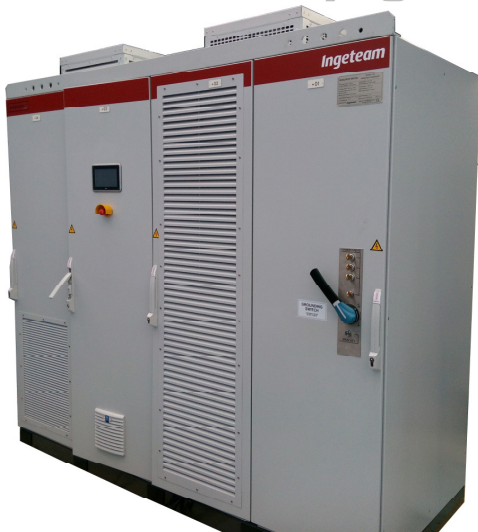
Fig. 15. 5L-MPC B2B converter based 6.6 kV-1.5 MW prototype.
