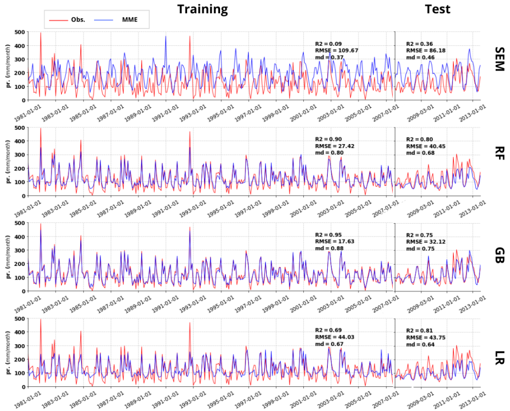
FIGURE 5.4: Spatially averaged observed precipitation and simulated precipitation time series and evaluation metrics (SEM and ML-MME) for the training (1980–2006) and test (2007–2015) periods.
