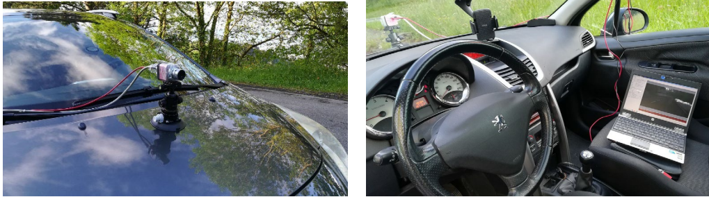
Fig. 1: The Photonfocus camera mounted on the front hood of the vehicle (top) and the recording laptop inside the car (bottom).
