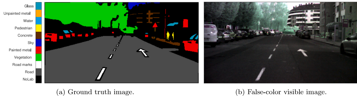
Fig. 1. Ground truth image (a) and its corresponding false-color visible image (b) of an urban scenario as an example of the weak labeling methodology followed to develop the HSI-Drive dataset. (For interpretation of the references to color in this figure legend, the reader is referred to the web version of this article.)
