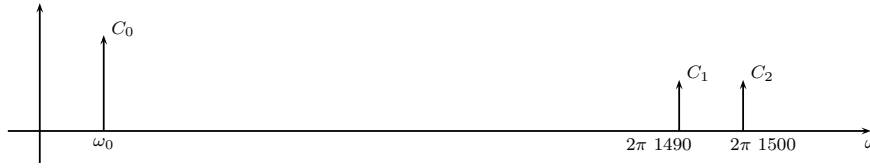
Figure A.7: Frequency diagram of the u_1(t) signal, output of flickermeter Block 1.
