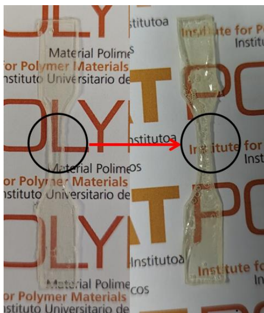
Figure 25. Appearance of the bubbles in the probe after curing.
