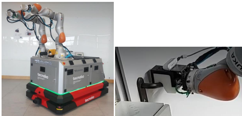
Fig. 1. Robot (AIMM) used in the tests, together with the gripper used for door opening.
