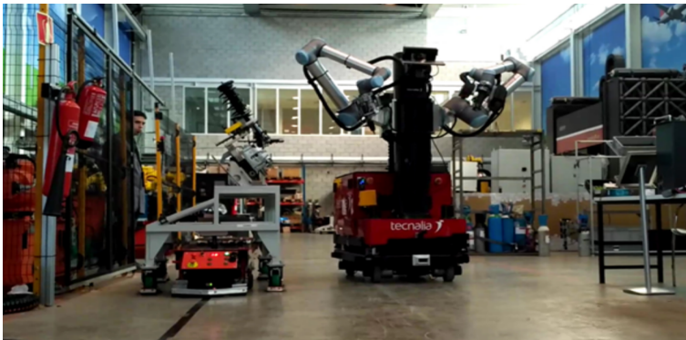
Figure 13. MRP following the mobile product platform (MPP) through the dynamic docking (visual servoing) system.
