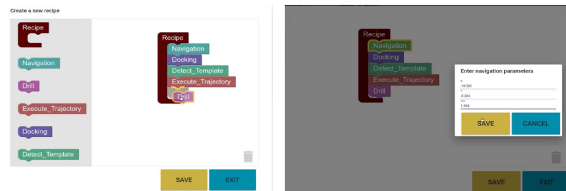
Fig. 4. Graphical interface developed for the creation and parameterization of a list of skills learned by the robot.
