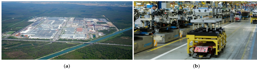
Figure 2. PSA facilities. (a) An aerial view of the plant. (b) One of the automatic guided vehicles (AGVs) of the plant transporting assembly pieces. ©PSA.
