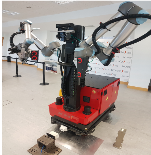
Figure 1. The Mobile Robotic Platform (MRP) navigating autonomously to the charging station.
