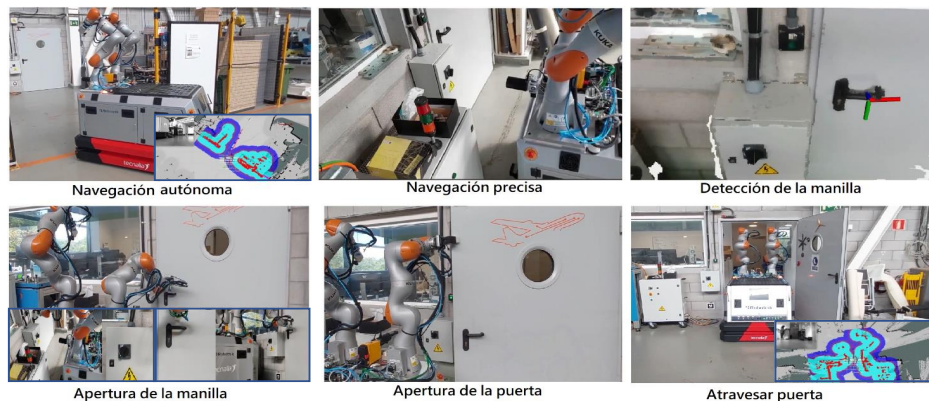
Fig. 5. Task execution flow for door opening.
