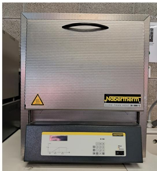
**Figura 103. Horno Nabertherm B180**
