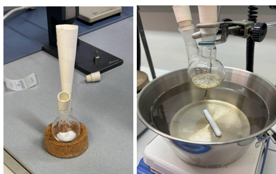
Figure 13. Flask containing PLEB 8020 and submerged in oil bath
