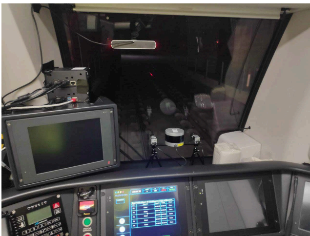
FIGURE 2. Camera setup for CAF dataset, placed in the cabin of a train moving through an underground urban railway scenario.
