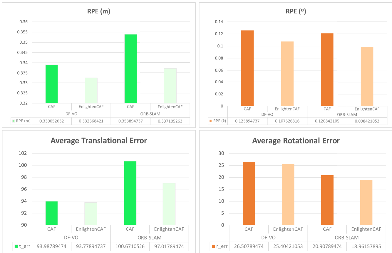
FIGURE 13. Comparison of relative VO evaluation metrics when applying DF-VO and ORB-SLAM2 algorithms in CAF and EnlightenCAF datasets. Translational and rotational components of relative errors are shown separately.
