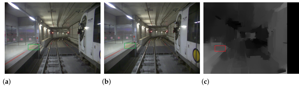
Figure 5. Distance calculation to platform landmark using stereo vision camera (left (a) and right (b) images) and extracted depth map (c). Green frames represent detected landmark bounding box and the red frame the landmark's corresponding area in depth map. This area is used for distance calculation.
