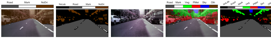
Fig. 8. Image 228 (f8, AG1, 10ms), captured during a spring, sunny midday, in an urban environment with shadows: (far left) Exp1 segmentation, (left) Exp1 ground-truth, (center) false color, (right) Exp3 segmentation and (far right) Exp3 ground-truth.
