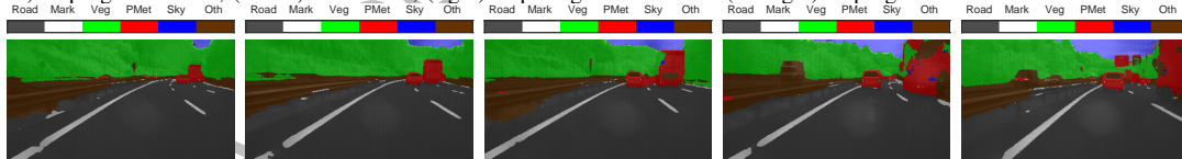
Fig. 5. Segmentation of video sequence 752, captured during a winter, rainy morning, in highway under adverse lighting and weather conditions. The time difference between every two frames is 3s.
