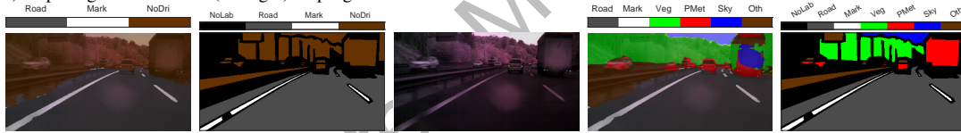
Fig. 4. Image 752 (f8, AG2, 20ms), captured during a winter, rainy morning, in highway under adverse lighting and weather conditions: (far left) Exp1 segmentation, (left) Exp1 ground-truth, (center) false color, (right) Exp3 segmentation and (far right) Exp3 ground-truth.
