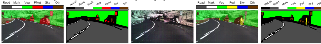
Fig. 9. Image 404 (f8, AG1, 10ms), captured during a fall, sunny midday, in road with Painted/Unpainted metal objects with similar shape: (far left) Exp3 segmentation, (left) Exp3 ground-truth, (center) false color, (right) Exp4 segmentation and (far right) Exp4 ground-truth.
