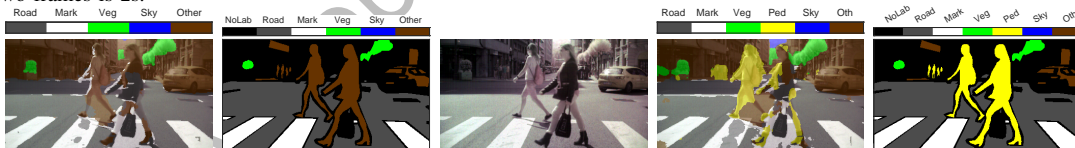
Fig. 13. Image 229 (f8, AG1, 10ms), captured during a spring, sunny midday, in urban environment with two pedestrians in a zebra crossing: (far left) Exp2 segmentation, (left) Exp2 ground-truth, (center) false color, (right) Exp4 segmentation and (far right) Exp4 ground-truth.
