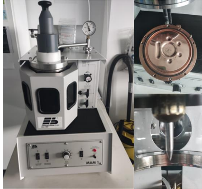
Figure 2.2. Edmund Bühler Compact Arc Melter MAM-1, cooper surface and tungsten tip used for the polycrystalline alloys re-melting and homogenization.
