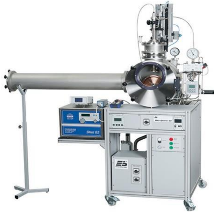
Figure 2.3. Edmund Bühler Melt Spinner MSP10. Figure taken from 9
