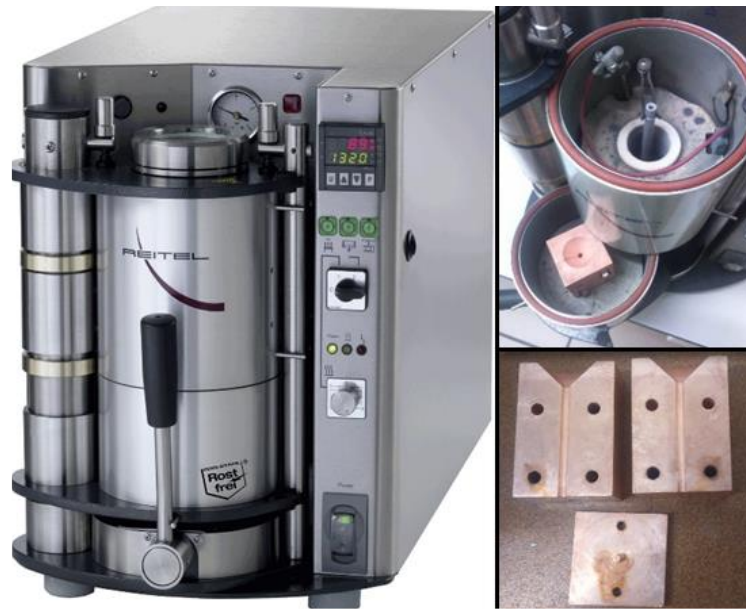
Figure 2.1. Reitel Induret Compact induction furnace, crucible and cooper mold used for polycrystalline rods production. Figure taken from 3
