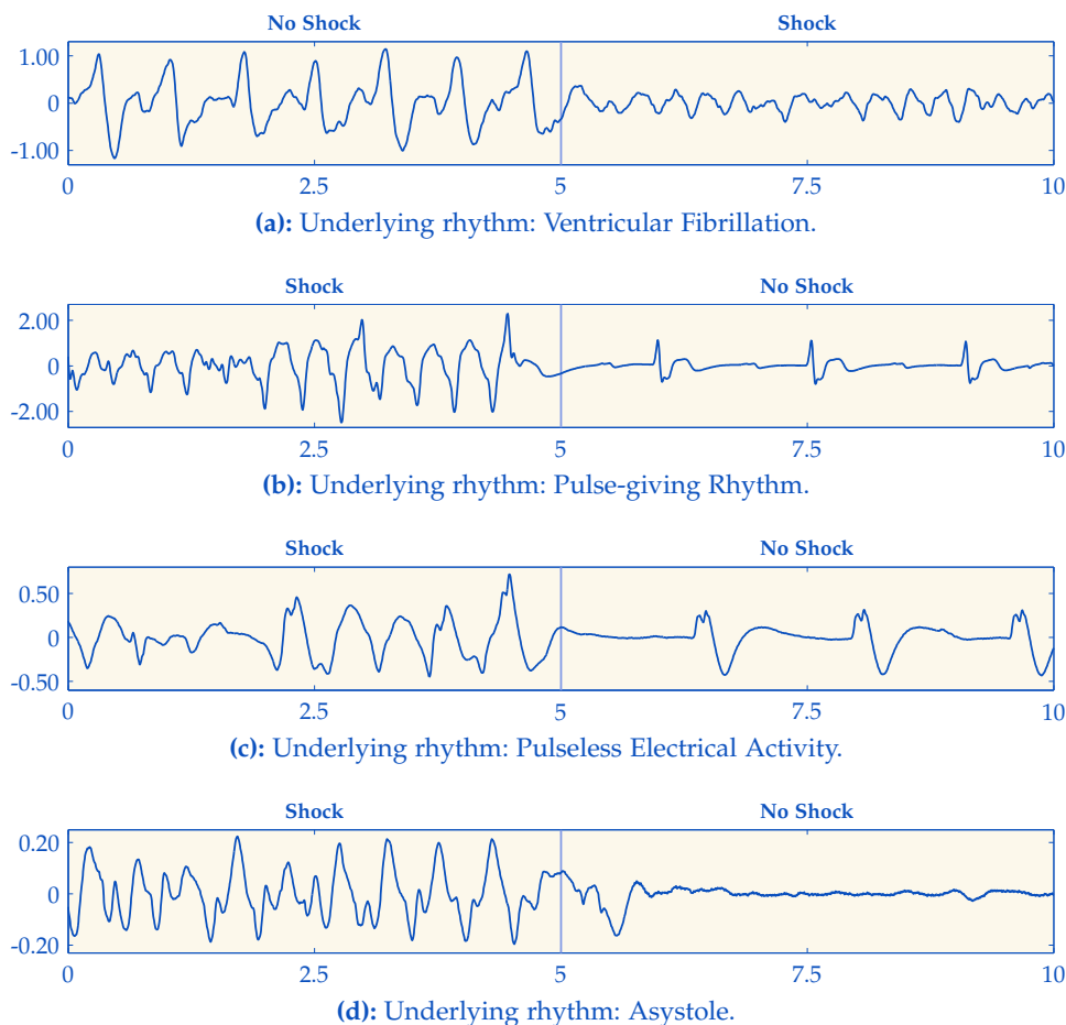
Figure 2.4: Examples of CPR artifact in OHCA episodes. During the initial 5 s, the CPR artifact corrupts the ECG. During the following 5 s, CPR is stopped, and the recorded signal shows the underlying heart rhythm. The shock/noshock decisions with and without CPR artifact show how a direct analysis of the corrupted ECG is not reliable (the real analysis interval is longer than 5 s). The y axis shows the ECG in mV.
