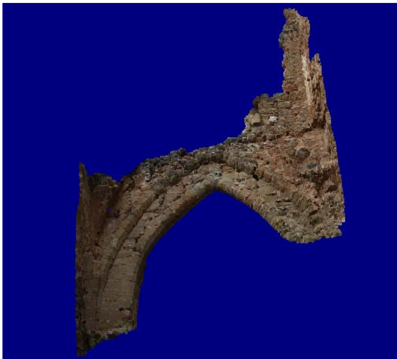
Fig. 2. Point cloud of the western wall
