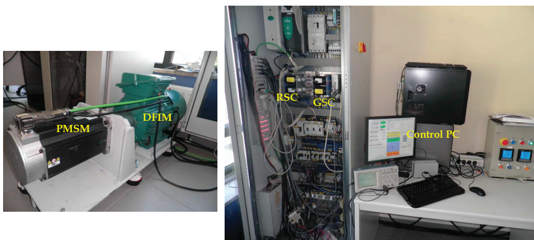
Figure 4. Photography of the DFIG wind turbine experimental platform.
