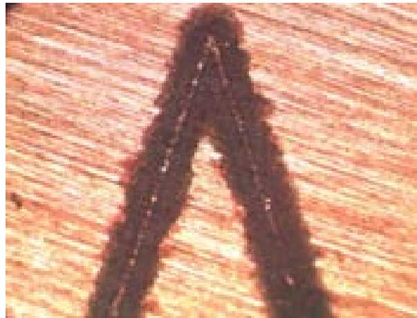
Figure 5.13. Thermal damage on OFE surface caused by a bad selection of laser parameters.
