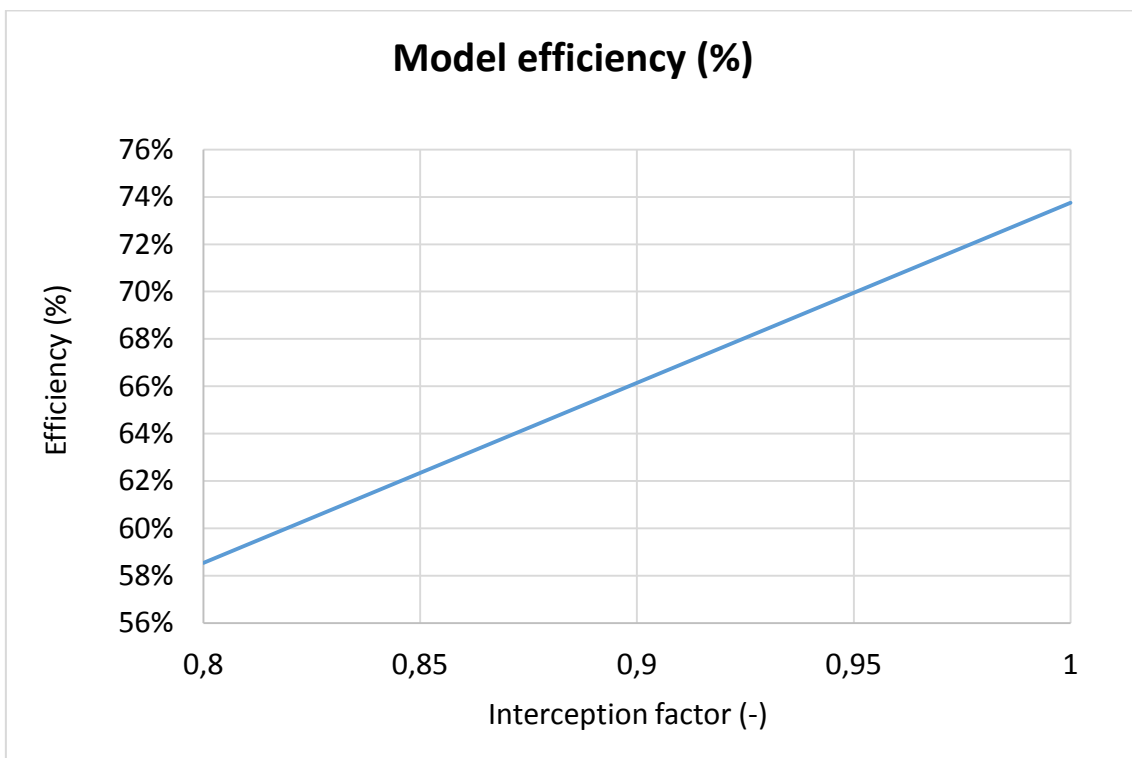
Figure-A 52. Graphs of the results for the dynamic efficiency test when the interception factor of the collector varies from 0,8 to 1.
