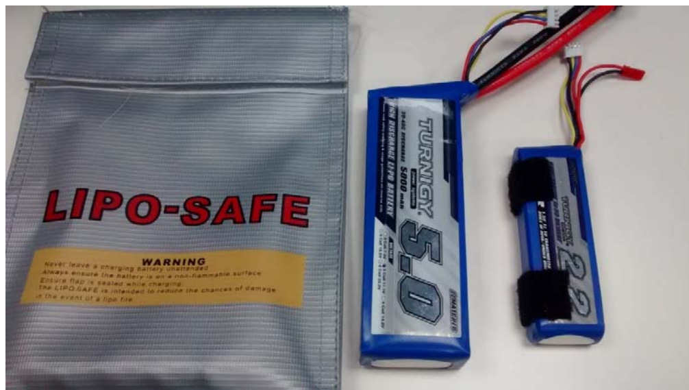
Fig 5: Left, fire resistant safe bag to store Li-Po batteries. Middle, 5000 mAh 3S battery pack for our quadrotor. Right, 2200 mAh 3S battery for the radio transmitter.
