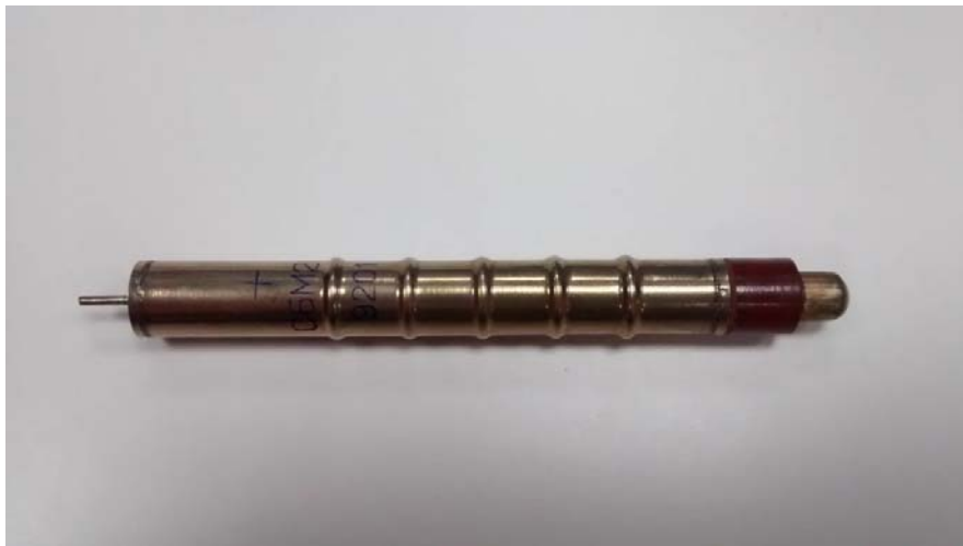
Fig 15: Image of the SBM20 a Russian Geiger-Muller tube. To the left the small tip of the Anode is isolated from the external wall (Cathode).
