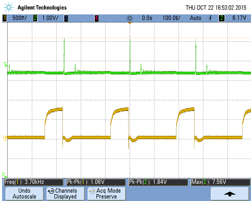
Fig 23: Measurements done on the Geiger circuit. One probe (yellow) measures the voltage on the switching transistor gate (T2). The green signal is measured through a 1GOhm resistor to dampen the signal 100 times. Once the transistor shuts inductor supply we see an immediate voltage kickback.
