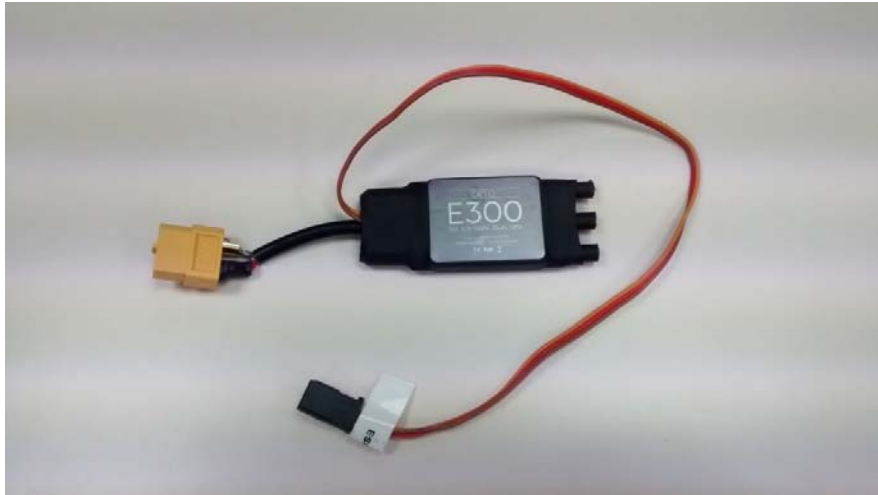
Fig 2: E300 electronic speed controller. Battery feeds through XT-60 connectors (Yellow). The 3 pin connector drives the PWM signal from the flight controller.
