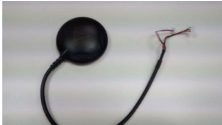
Fig 9: The GPS module, LEA-6H GPS, contains a GPS and a compass. The compass is very useful as we can separate the GPS module from noise sources like motors.
