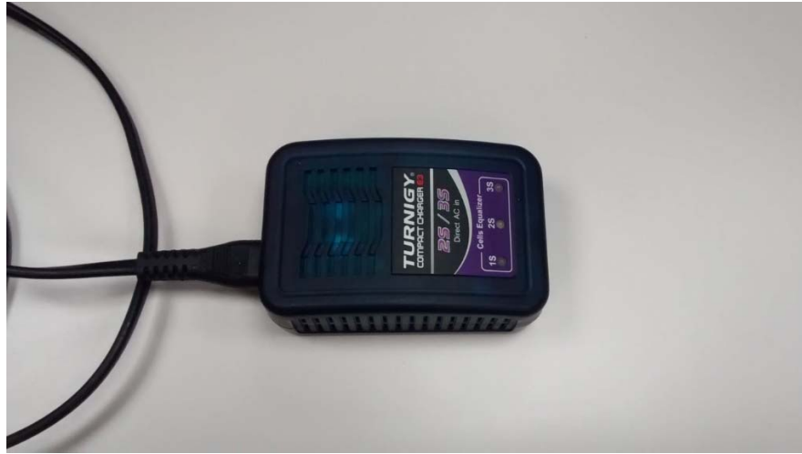
Fig 6: Basic Li-Po charger. Can charge 1S, 2S and 3S battery packs.
