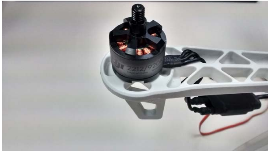
Fig 3: 2212 brushless motors connected by 3 bullet connectors to the ESC's. Four screws hold it to the frame (White). The ESC ( under the frame arm ) will be tied to the arm with bridles.
