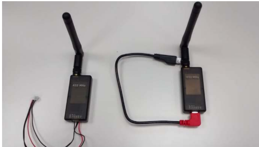
Fig 8: Radio transmitter and receiver (With antennas). Left, DF13 connector goes to the APM telemetry port. Right, connected via USB to the PC.
