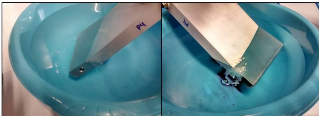
Figure 6-13: Bubbling produced in a closing system with a leak (right) vs. a suitable airtight plate (left)
