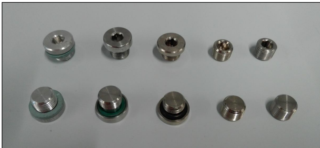
Figure 6-11: Some types of the tested threaded plugs. From left to right: aluminum headed plug with flat paper gasket; stainless steel headed plug with Viton O-ring gasket; brass headed plug with Viton O-ring gasket, brass non-headed plug and stainless steel non-headed plug
