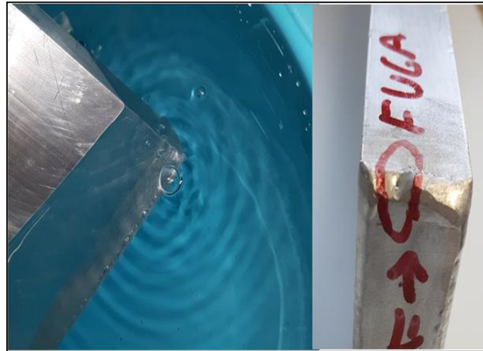
Figure 6-14: Leak produced by deficient welding
