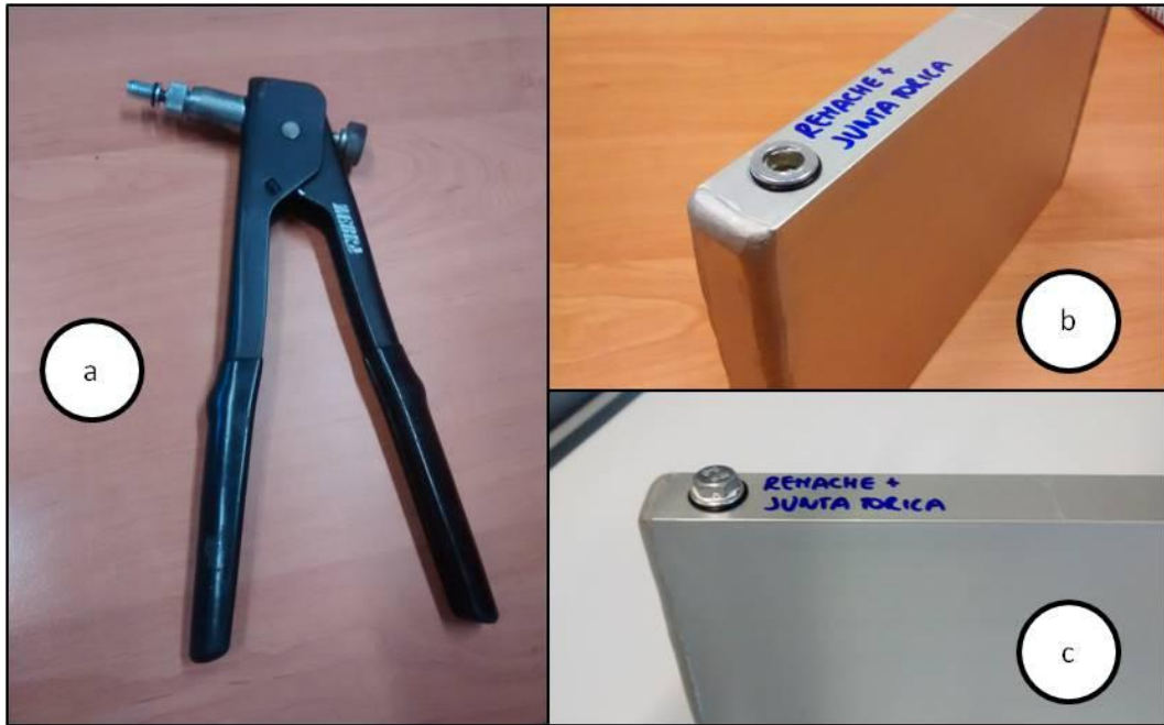
Figure 6-9: a) Rivet gun; b) Plate with a rivet nut inserted; c) Plate with a rivet nut inserted and closed with a threaded screw
