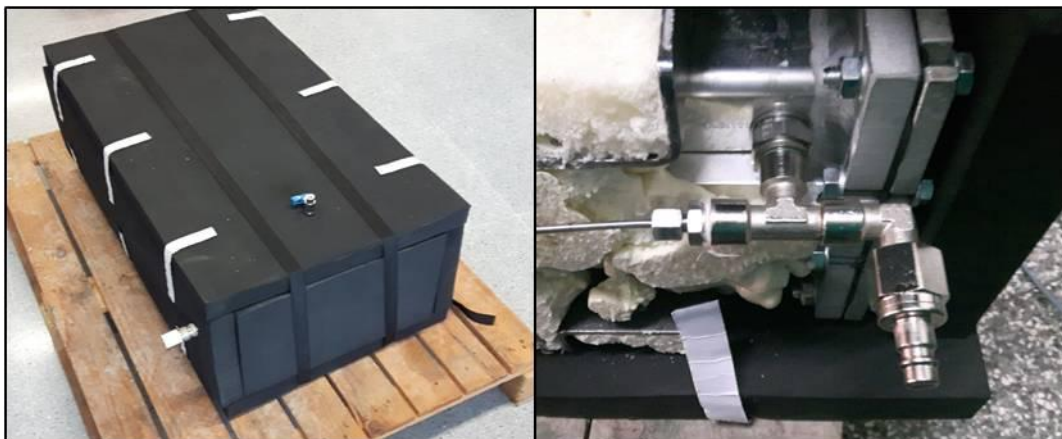
Figure 6-8: Outer aspect of the tested LHTES prototype with the insulation (left) and detail of the HTF inlet hydraulic connection (right)
