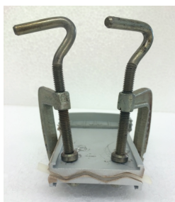
Figure 6.6. Employed home-made gadget to deform the sample.
