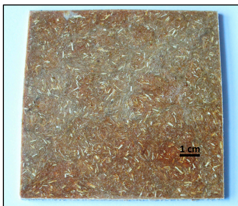
Figure 1. Chicken feather/PLA biocomposite containing 50 wt % of feather.
