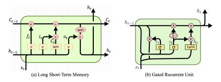
Figure 7: Schemes of LSTM and GRU unit-types<sup>7</sup>
