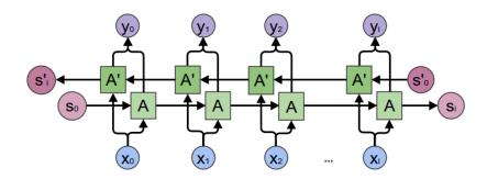
Figure 6: Example of a bidirectional RNN<sup>6</sup>
