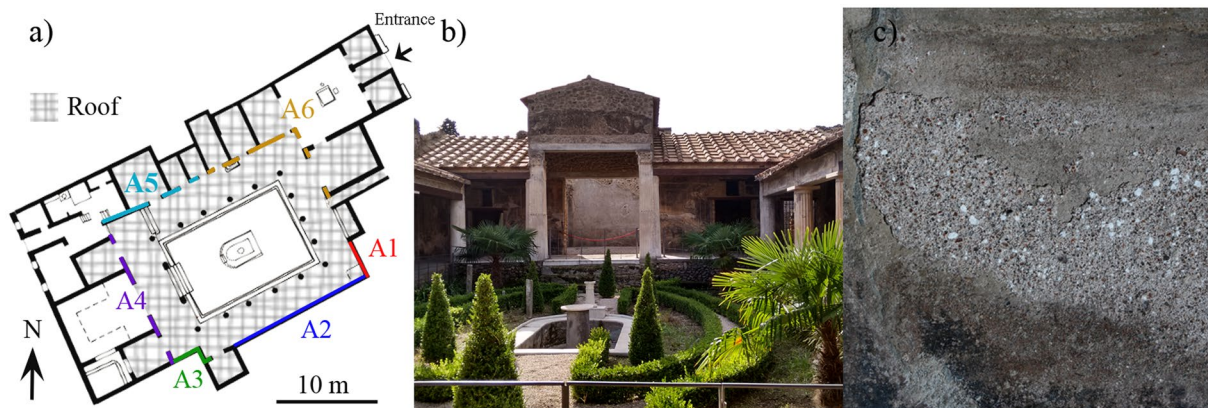
Figure 1. (a) Plan of the House of Gilded Cupid (Pompeii) showing the different measured areas (A1-A6). (b) Recent photograph of the wooden roof dated from 2004 that covers the wall paintings of the peristyle. (c) Detail of the sub-efflorescences formed in the intonaco in one of the studied walls.
