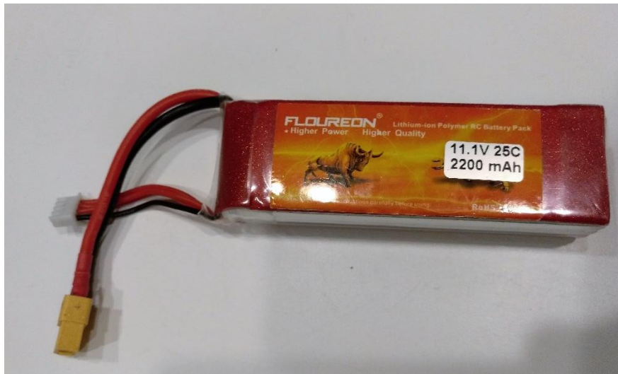
Figure 25: Battery with 11.1 V DC output
