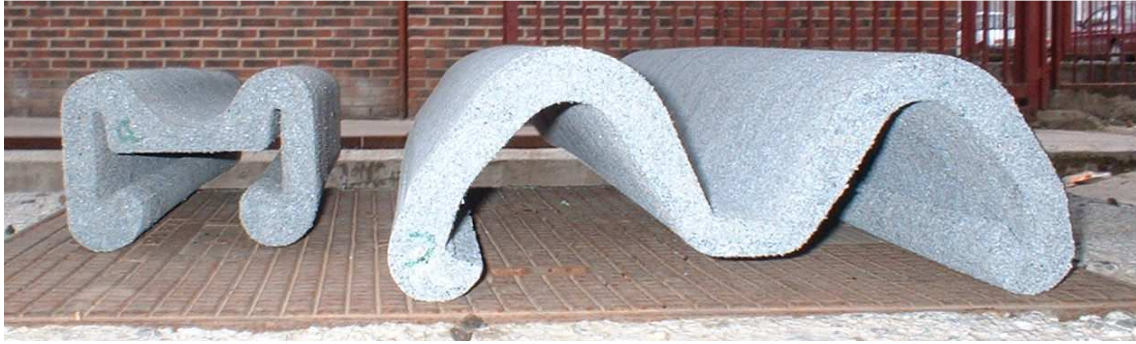
Fig. 2-1 Sample of recycled rubber and Linear Low Density Polyethylene blend with the shape of crash barrier and poles
