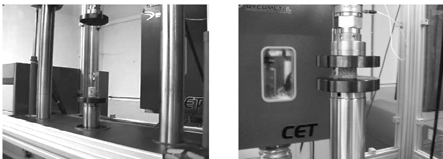
Fig. 3-9 MTS High Rate Test System at mechanical testing laboratory of LEARTIKER
