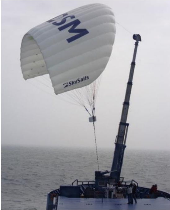
Figure 2.2. Kite sail rope on the Theseus (SkySails, n.d.)
