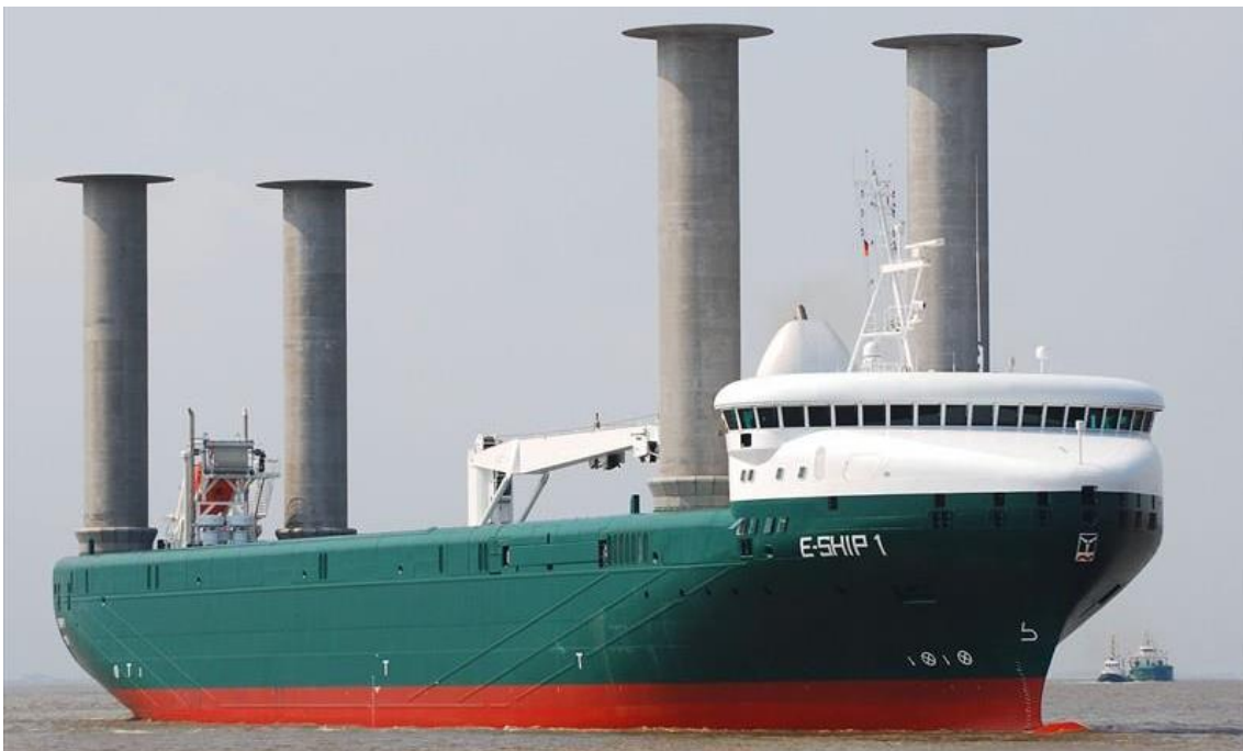
Figure 2.7. E-Ship 1 with Flettner Rotors on her deck (Marine Insight, 2013).
