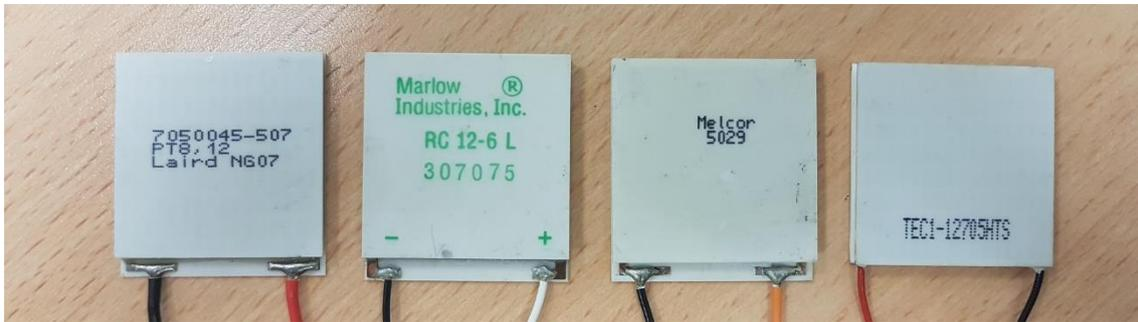
Fig. 12. Celdas Peltier de Laid Technologies [21], Marlow Industries [22], Melcor [23] , y Hebeild [24]
