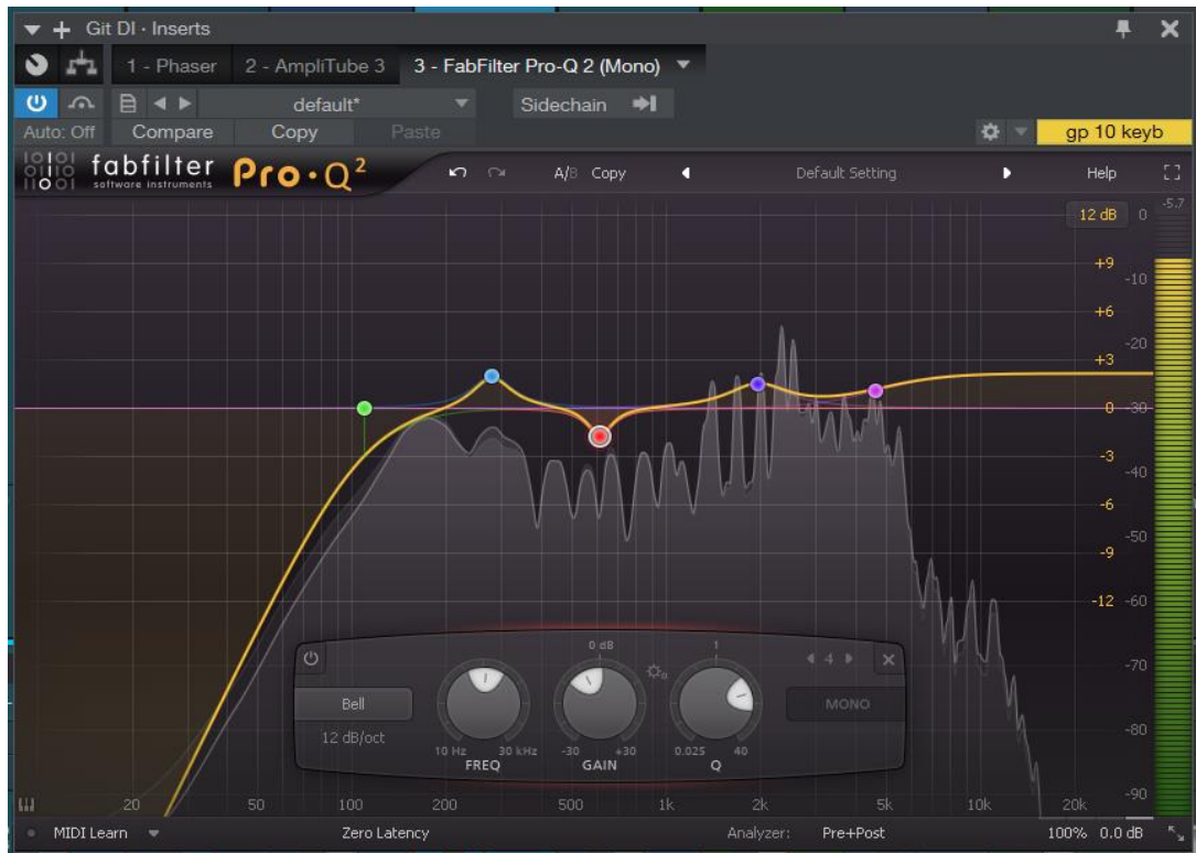
Figure 8: Equalizer showing natural voice wave. In its complexity, many frequencies resonate, and the equalizer tries to shape and improve the audio by manipulating those harmonics
