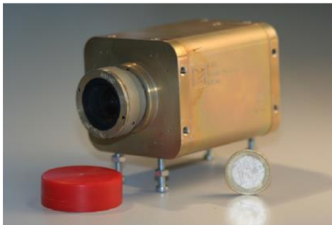
Figure 2. A VMC unit with the protective lens removed and 1 euro for size comparison [3].
