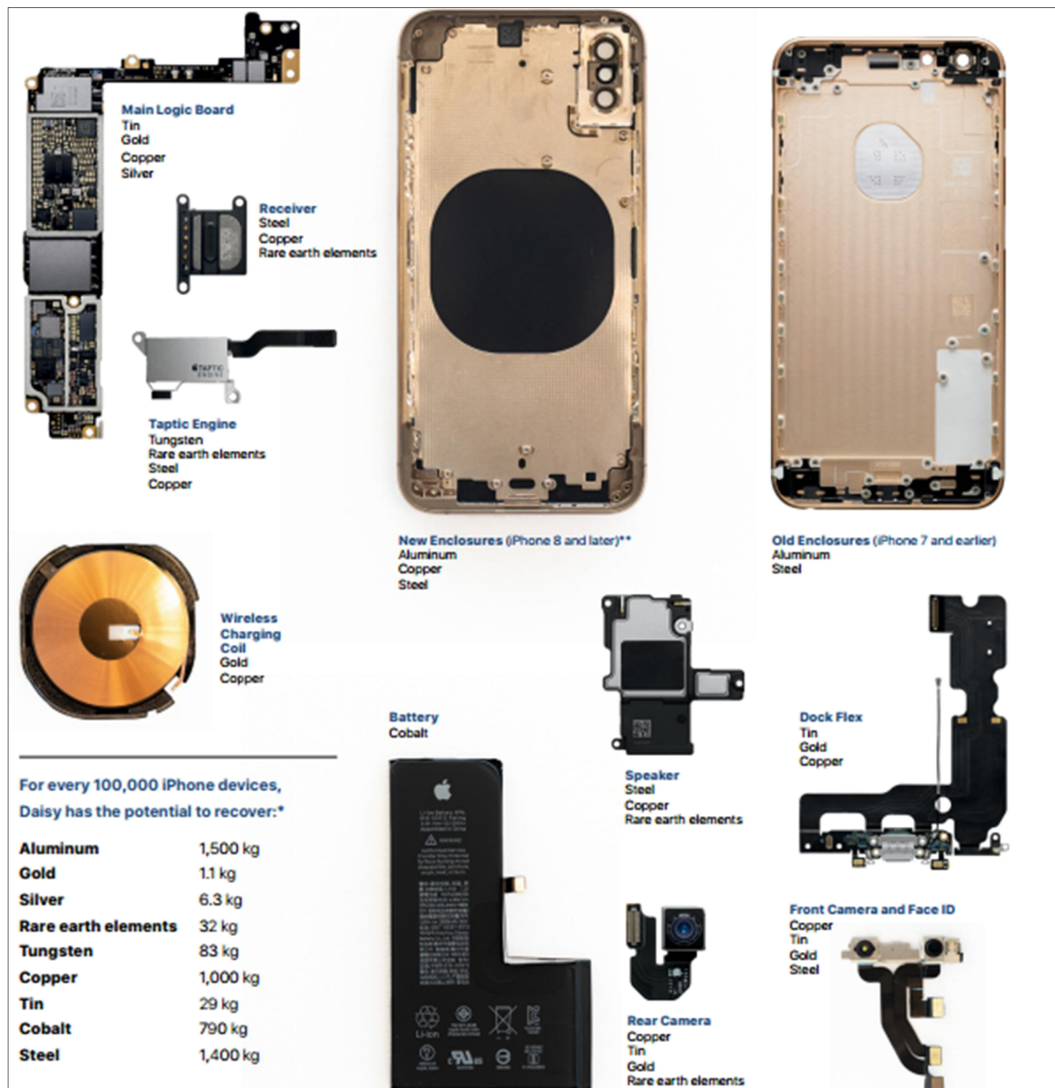
Figure 20: Components and materials disassembly robot Daisy recovers [81]
