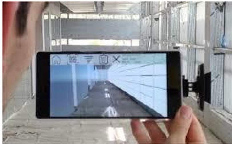
Figure 18: AR4C application used in construction site [75].
