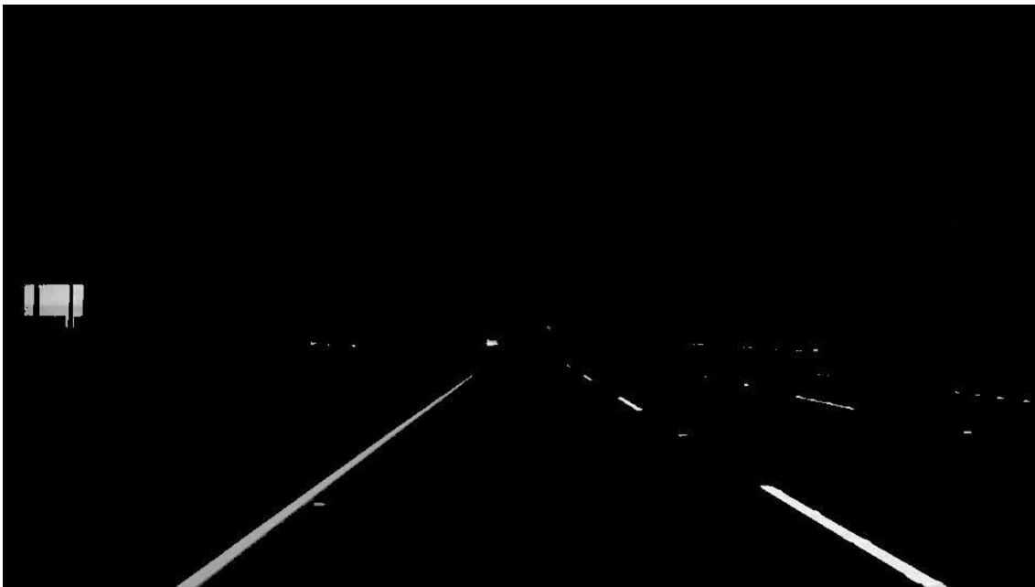
Figure 10: Image of road after isolation of white color
