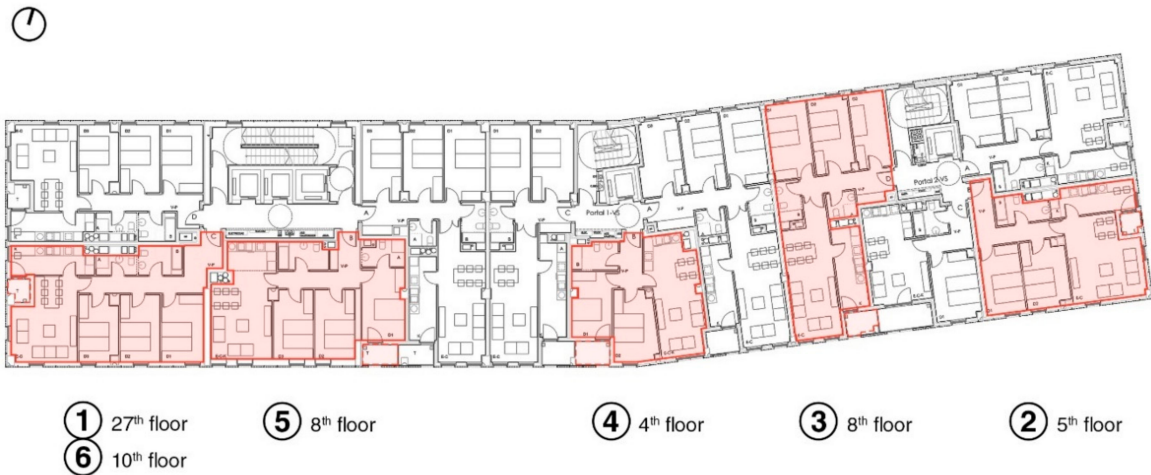
Figure 3. Typical floorplan of the Bolueta Tower. The monitored apartments are highlighted in red, with indication of the storey. The western third (left in the image) rises to 27 floors, while the remaining two thirds have 9 floors. Source: Authors.
